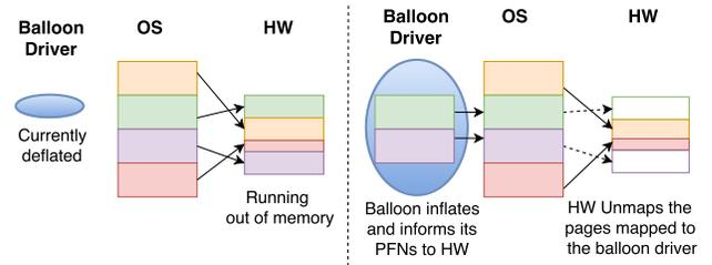
Fig. 8: Ballooning for OS-transparent handling of out-of-memory.
